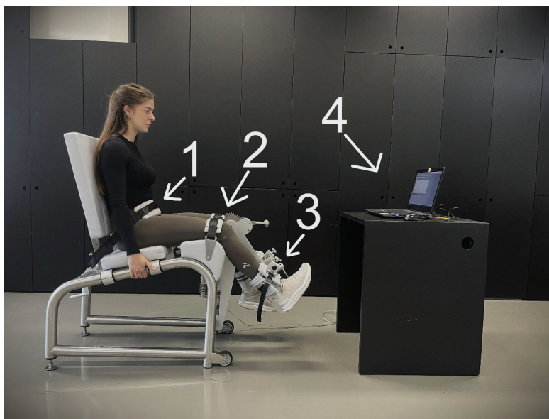
FIGURE 1. Position of the subject during the measurement of RFD-SF. 1 = a padded fixation of the pelvis; 2 = rigid straps for the knee fixation; 3 = force sensors; 4 = a monitor with visual feedback.
